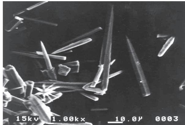
Fig. 11a. SEM photograph of scale formed in boiler wall in run 1.
