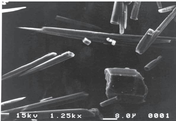
Fig. 10a. SEM photograph of scale formed on boiler wall during run 1.
