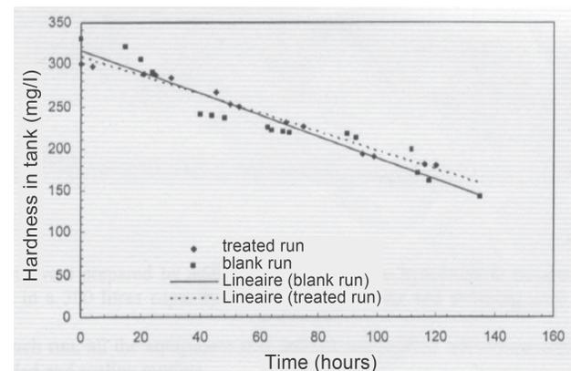
**Fig. 2. Depletion of hardness in treated and untreated regimes.**
