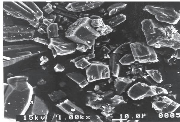
Fig. 11b. SEM photograph of scale formed in element boiler in run 1.
