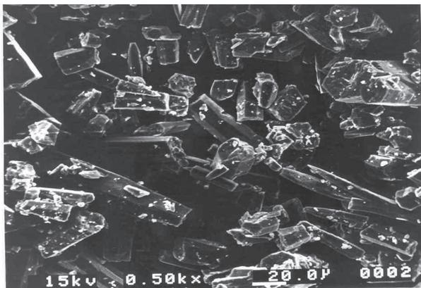
Fig. 10b. SEM photograph of scale formed on the element during run 1.
