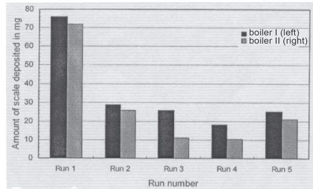
Fig. 7. The amount of scale deposited in both boilers.
