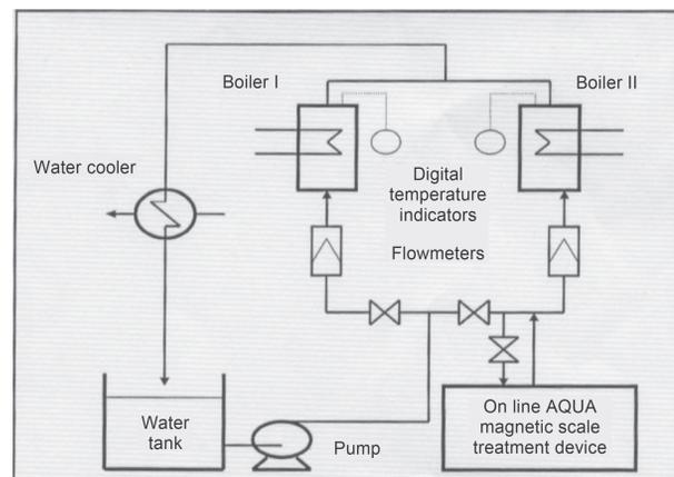
Fig.1. Schematic flowchart of the laboratory setup.
