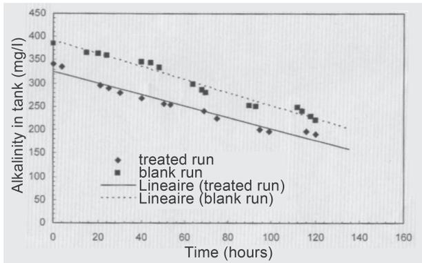
Fig. 3. Depletion of alkalinity in treated and untreated regimes.
