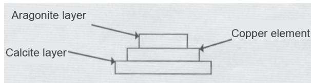
Fig. 12. Cross section of the scale deposits.
