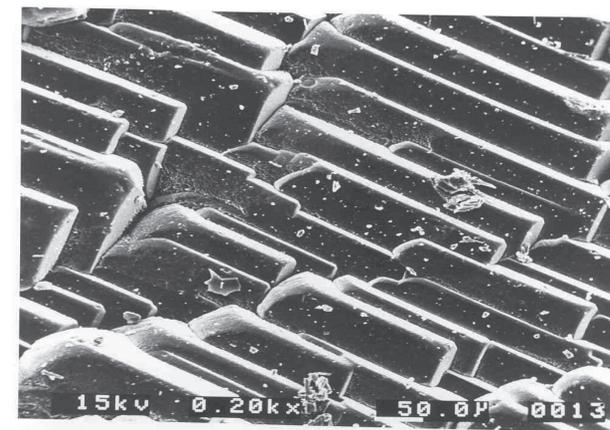
Fig. 9. SEM photograph of aragonite crystals deposited in a treated run.
