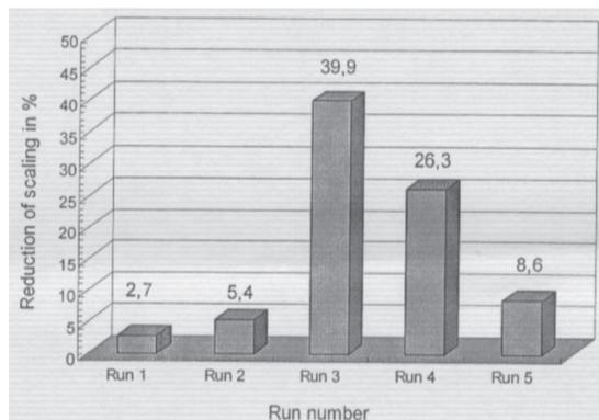
Fig. 6. The reduction of scale deposited in both boilers in %.
