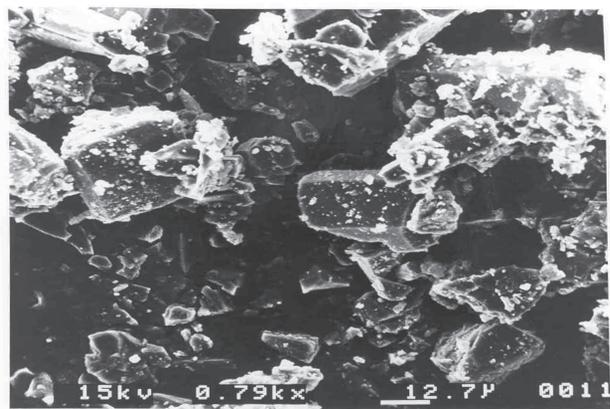
Fig. 8. SEM photograph of calcite crystals deposited in a treated run.
