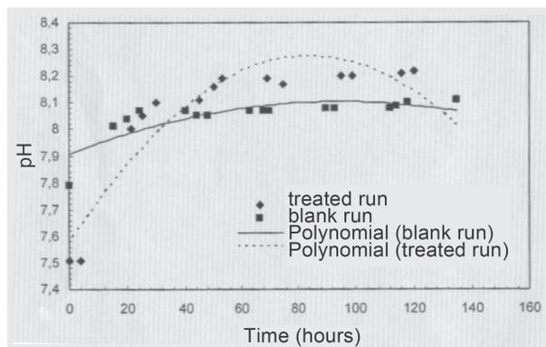
Fig. 4. Effect of the scaling on the pH.
