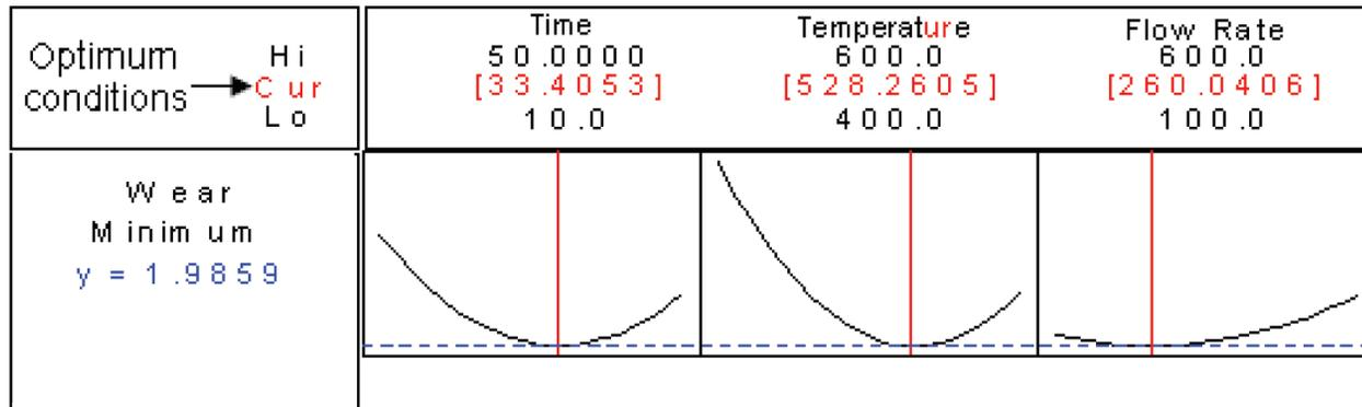
Fig. 10. Optimum nitriding conditions for minimum wear (1.9859 %).
