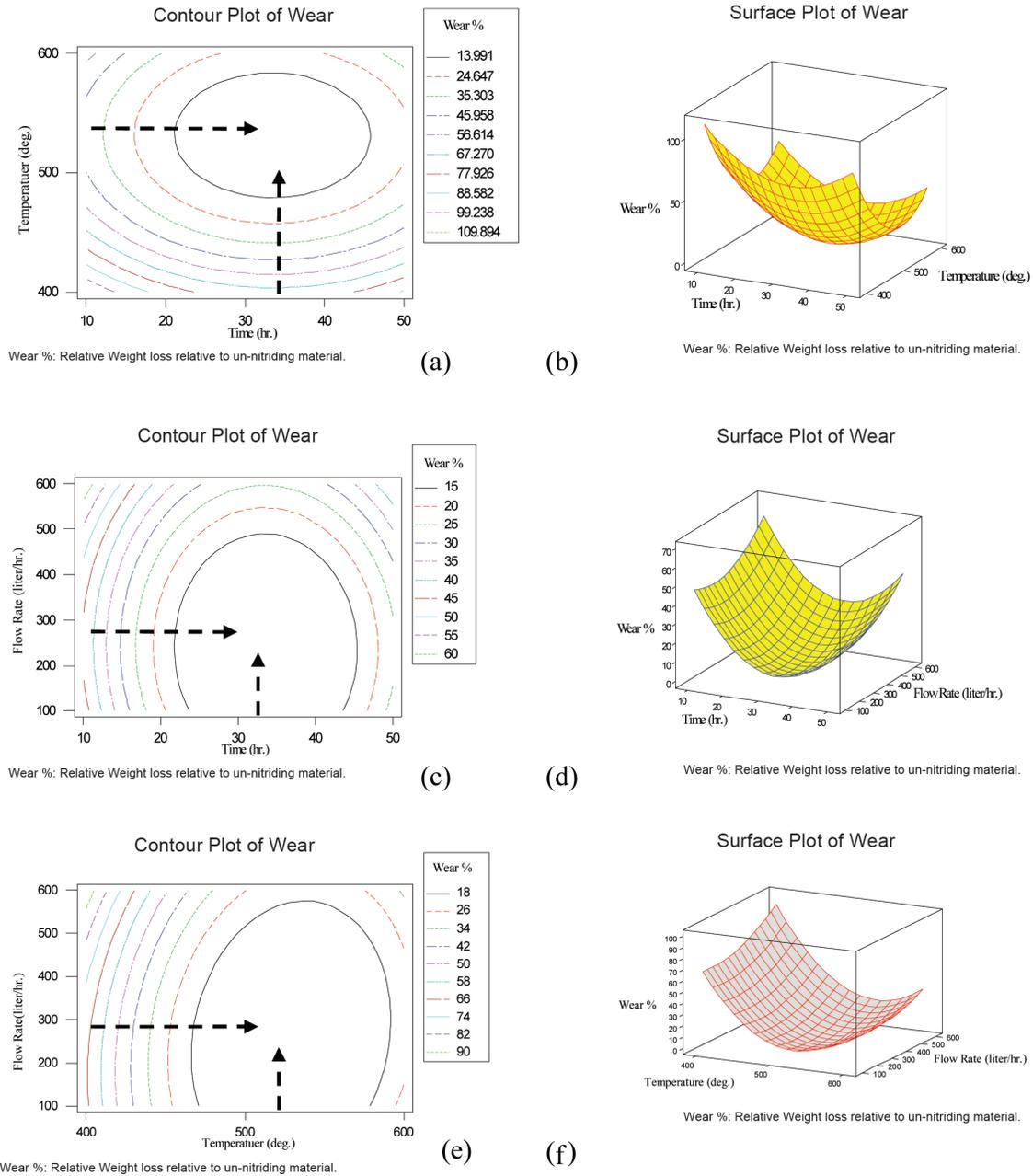
Fig. 9. Effects of nitriding processing parameters on wear resistance (MINITAB).
