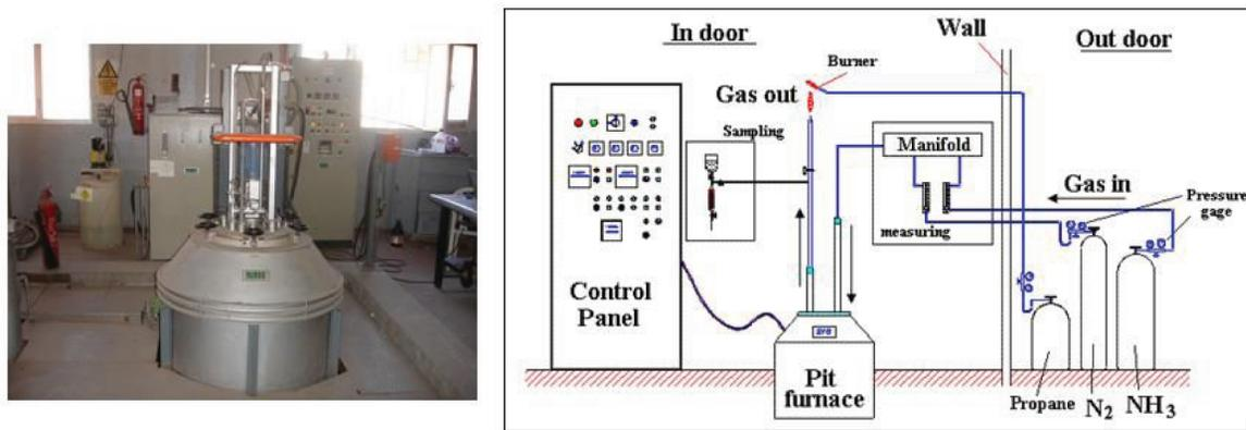
Fig. 4. The SIB Furnace (pit furnace type 752).
