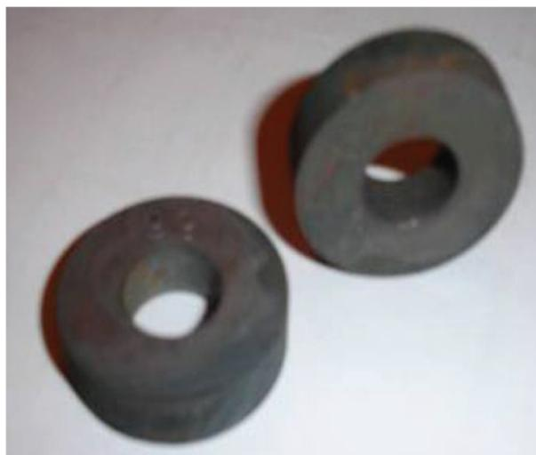
Fig. 3. Wear test specimen after nitriding.
