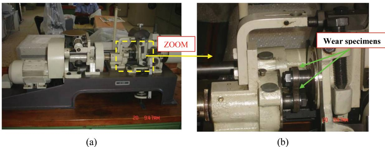
Fig. 5. Photographs showing an Amsler machine model A135 Wear Testing Machine, (a) overall shape of the wear apparatus, (b) zoomed to illustrate the specimens positions.
