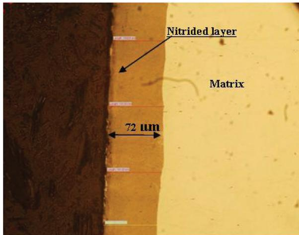
Fig. 6. Optical micrographs (OM) of a nitrided layer of AISI 316 (process No.1).
