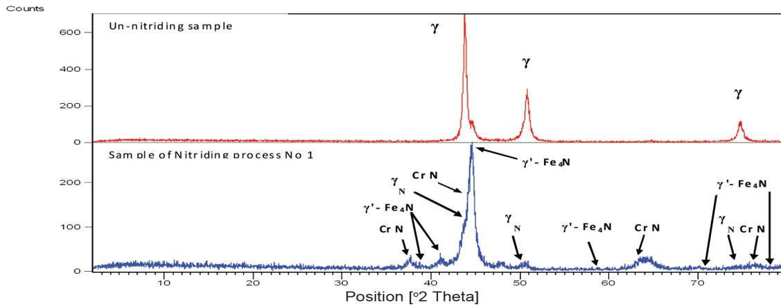
Fig. 8. X-ray diffraction patterns of a nitrided layer of nitriding process No. 1.
