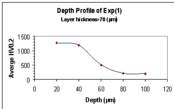
Fig. 7. Hardness profile across the nitrided layer (nitriding process No.1).
