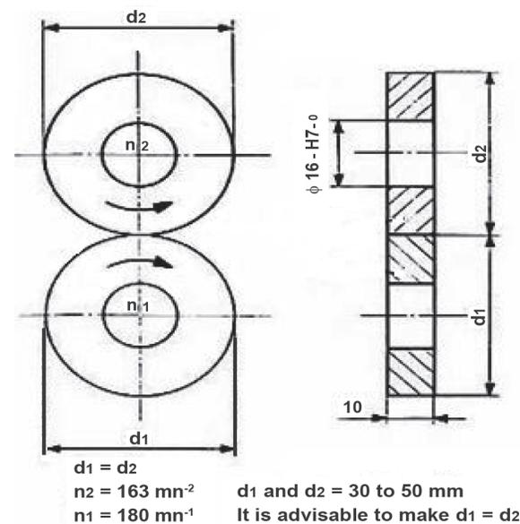
Fig. 2. Rolling and sliding wear test specimen's shape and dimensions.
