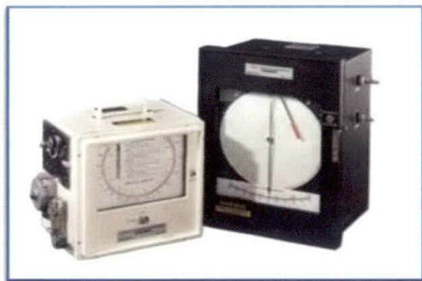
Fig. 7. Proptional Torque Differential indicator for measuring the specific gravity gas.
