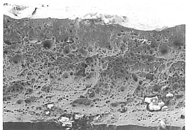
FIG. 2. S.E.M. fractography shows typical ductile fracture of stainless steel specimen fractured in air.
