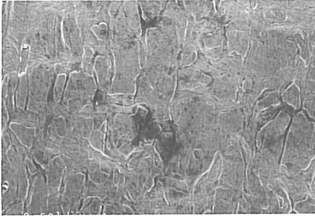
FIG. 11. S.E.M. micrograph of an 12% cold worked 304 austenitic stainless and specimen strained in solution at a crosshead of 9.8 nm/s. Micrograph shows very little surface cracks.
