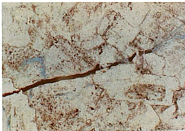
PLATE 4: Well: B2-102; Depth: 8822'6"; Lithology: GR; Porosity: 2% est.; Magnification: \times 64 .
