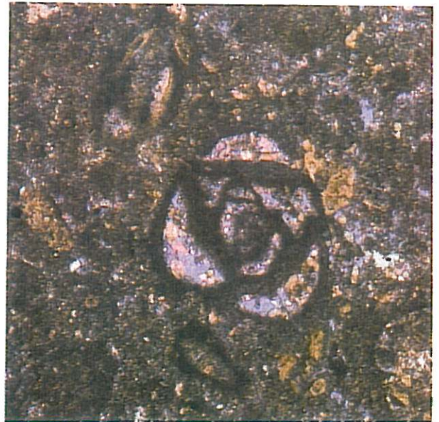
FIG. 4c. The Khalifa limestone also has a pore system dominated by micropores with isolated molds and vugs.
