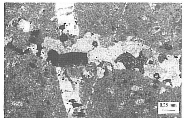
FIG. 12. Mudstone showing cross-cutting fractures represented by calcite veins. Note that some parts of the calcite vein are replaced by authigenic silica. Well E1-NC35A, XN.
