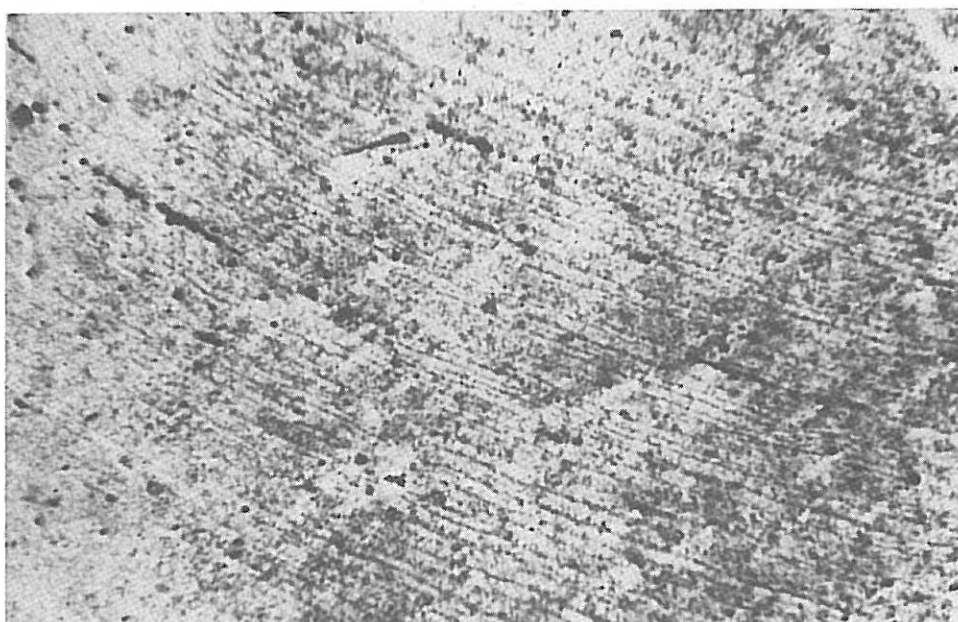
FIG. 6. Phosphorous segregation bands following the direction of plastic deformation in steel (E) Stead's reagent. Magnification 63 \times .
