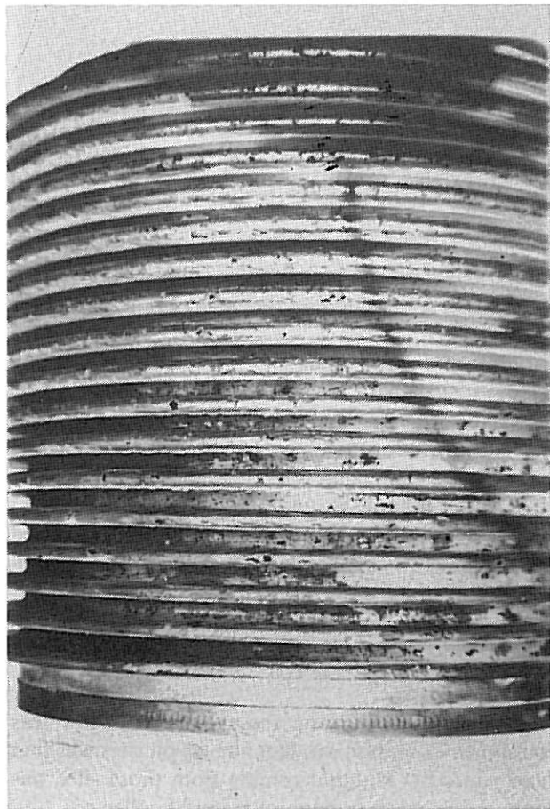
FIG. 1. Localized corrosion causing perforation.
