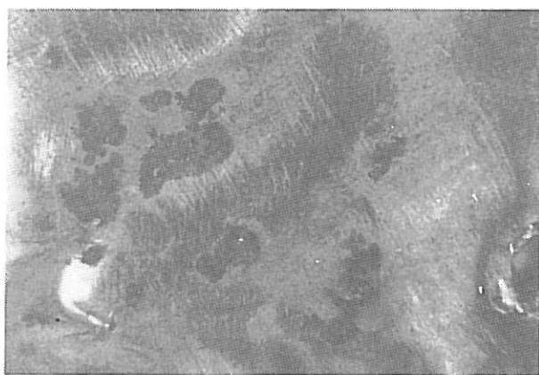
FIG. 5. Pitting caused by exposure to wet H 2 S above solution level X6.
