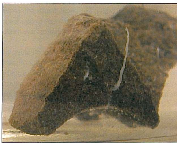
Fig. 1. Microbial contamination of preserved sample. A rock chip from a preserved sample which has been immersed in solvent. A stream of biopolymer can be seen eluting from the pore space. This sample was ruled unsuitable for formation damage testing due to bacterial contamination.
