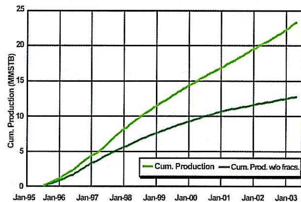
Fig. 8. Cumulative oil production Nakhla Oilfield with and without hydraulic fracs. Cumulative production without fracs obtained from well-by-well DCA.
