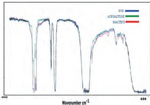
Fig. 7. IR spectra of the parent (BVR) and solvent extracted fractions.
