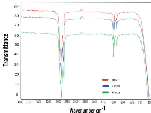
Fig. 8. IR spectra of the parent crude oils (Bouri, Sirtica and Breaga).
