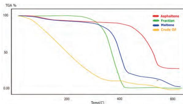
Fig. 6. TGA of Sirtica crude oil (SCO) and it's asphaltene (A), maltene (M) and vacuum residue Fraction (F).
