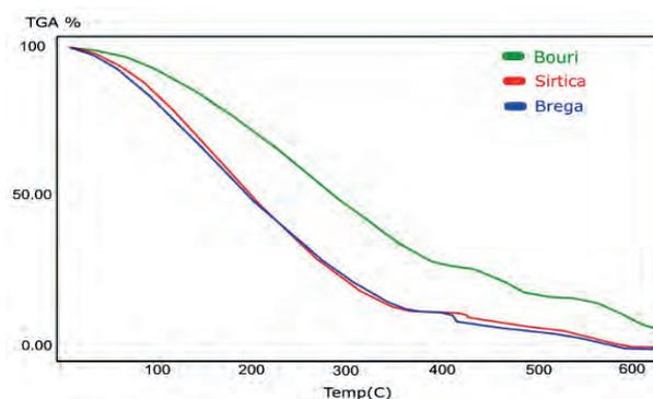
Fig. 3. TGA of the parent crude oils (Breaga, Sertica and Bouri).
