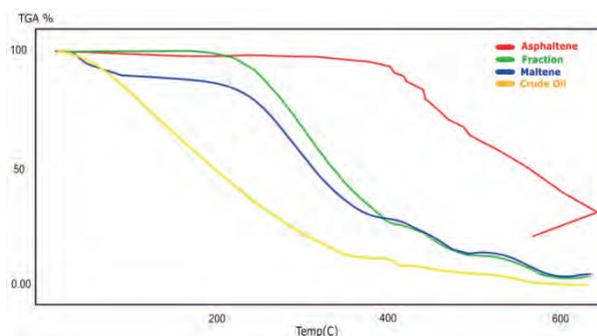
Fig. 5. TGA of Breaga crude oil (BrCo) and it's asphaltene (A), maltene (M) and vacuum residue (Fraction F).
