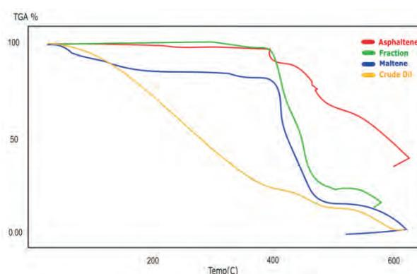
Fig. 4. TGA of Bouri crude oil (BCO) and it's asphaltene (A), maltene (M) and vacuum residue (Fraction F).
