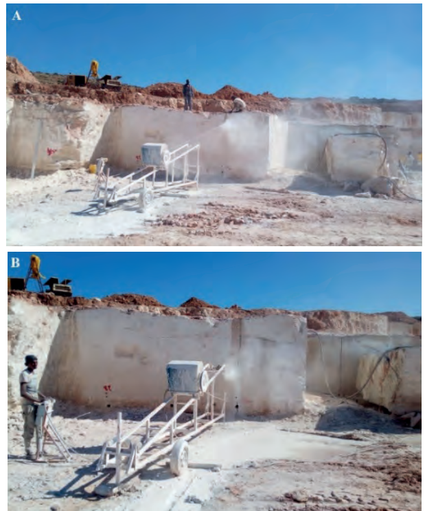
Fig. 3. Lateral cutting of a primary block with a diamond wire, a Libyan diamond wire saw machine. A) shows the beginning of cutting of the commercial block; B) the final stage of block separation.
