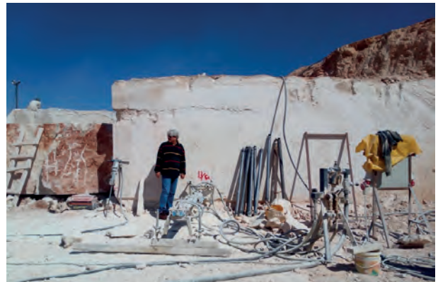
Fig. 2. The perforator drilling machine type for preparing drill holes for cutting the rock into commercial blocks using diamond wire.
