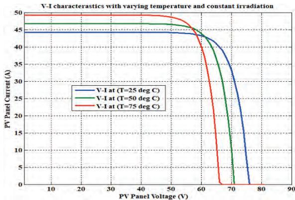
Fig. 5. V-I Characteristic curves at different cells working temperature (TC=25OC, 50OC, 75OC) for 6 module in parallel.
