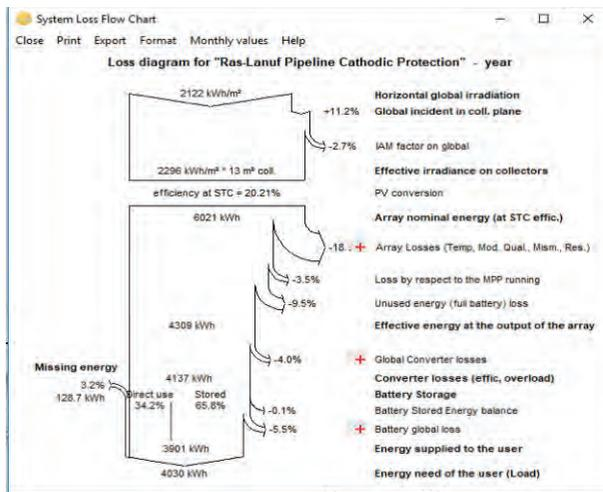
Fig. 10. System loss flow diagram.
