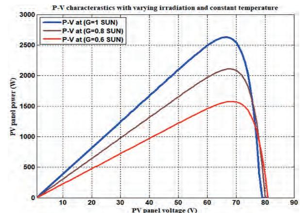
Fig. 4. P-V Characteristic curves at different insolation levels (G= 0.6 SUN, 0.8 SUN, 1 SUN) for 6 module in parallel.
