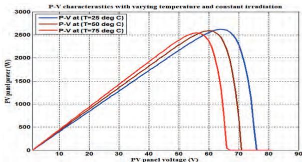
Fig. 6. P-V Characteristic curves at different cells working temperature (TC=25OC, 50OC, 75OC) for 6 module in parallel.
