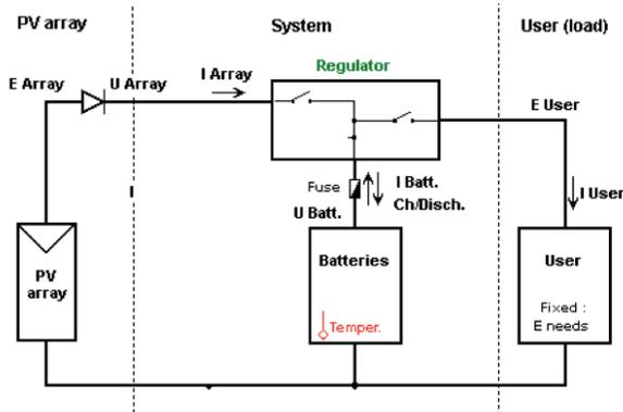
Fig. 9. Typical layout of PV system.
