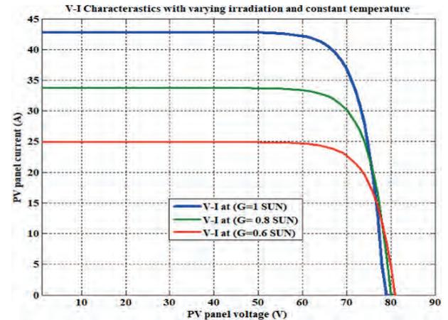
Fig. 3. V-I Characteristic curves at different insolation levels (G= 0.6 SUN, 0.8 SUN, 1 SUN) for 6 module in parallel.
