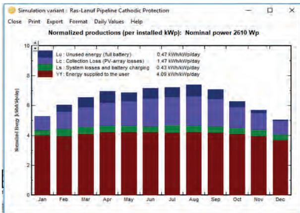
Fig. 11. Normalized production per installed KWP.
