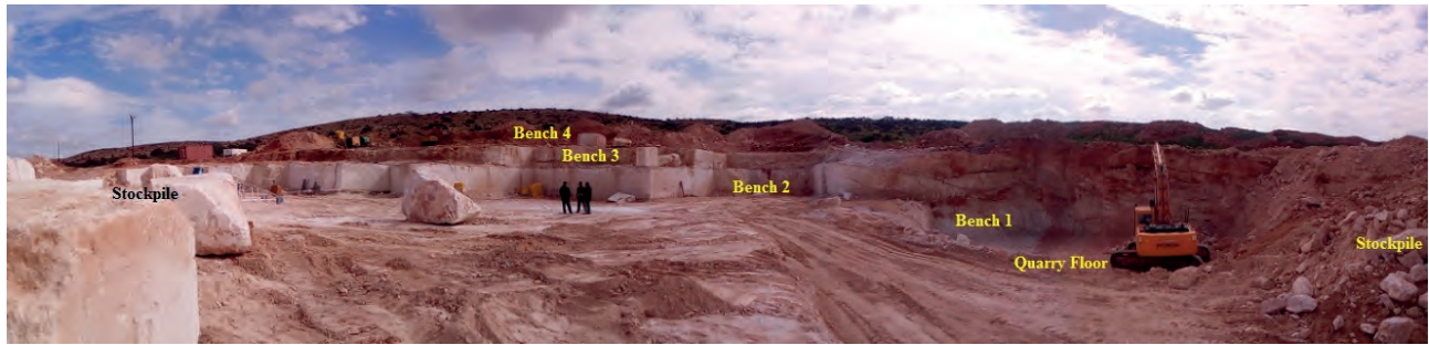
Fig. 6. Showing cut benches of Darnah Formation (looking, NE).
