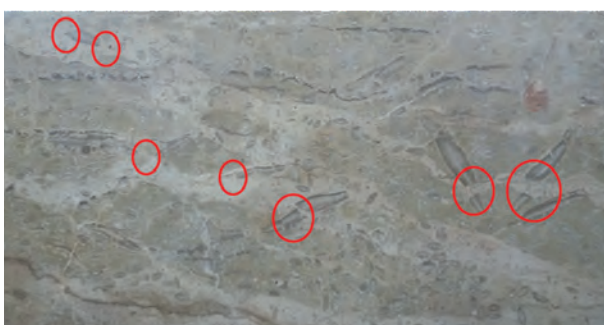
Fig. 9. A polished limestone of the uppermost the productive beds of bench (1) Nummulites shells are clearly affected by storm wave base (SWB) action.
