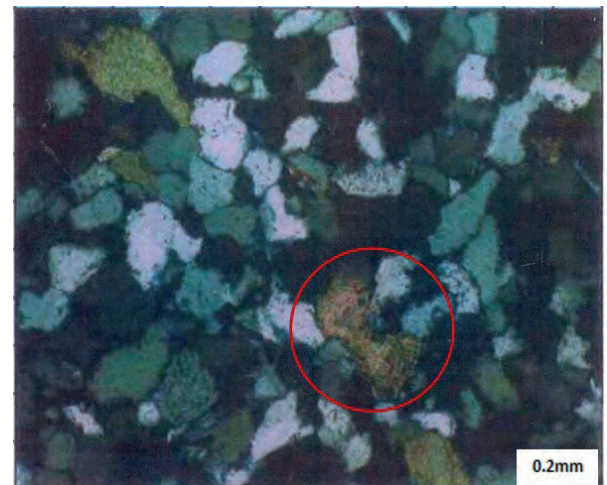
Fig. 14. Photomicrograph, showing pore-filling calcite cement within the Hawaz Sandstone, XPL, (X10).
