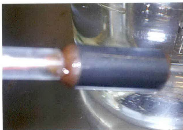
Picture 1 shows the iron oxide film formed as result of anodic polarization
