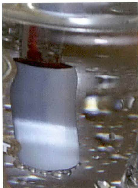
Picture. 2 Nice view of zinc hydroxide on steel Surface.
